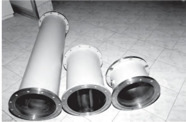
Fig. 5.6: Metal enclosures for GIS busbars
